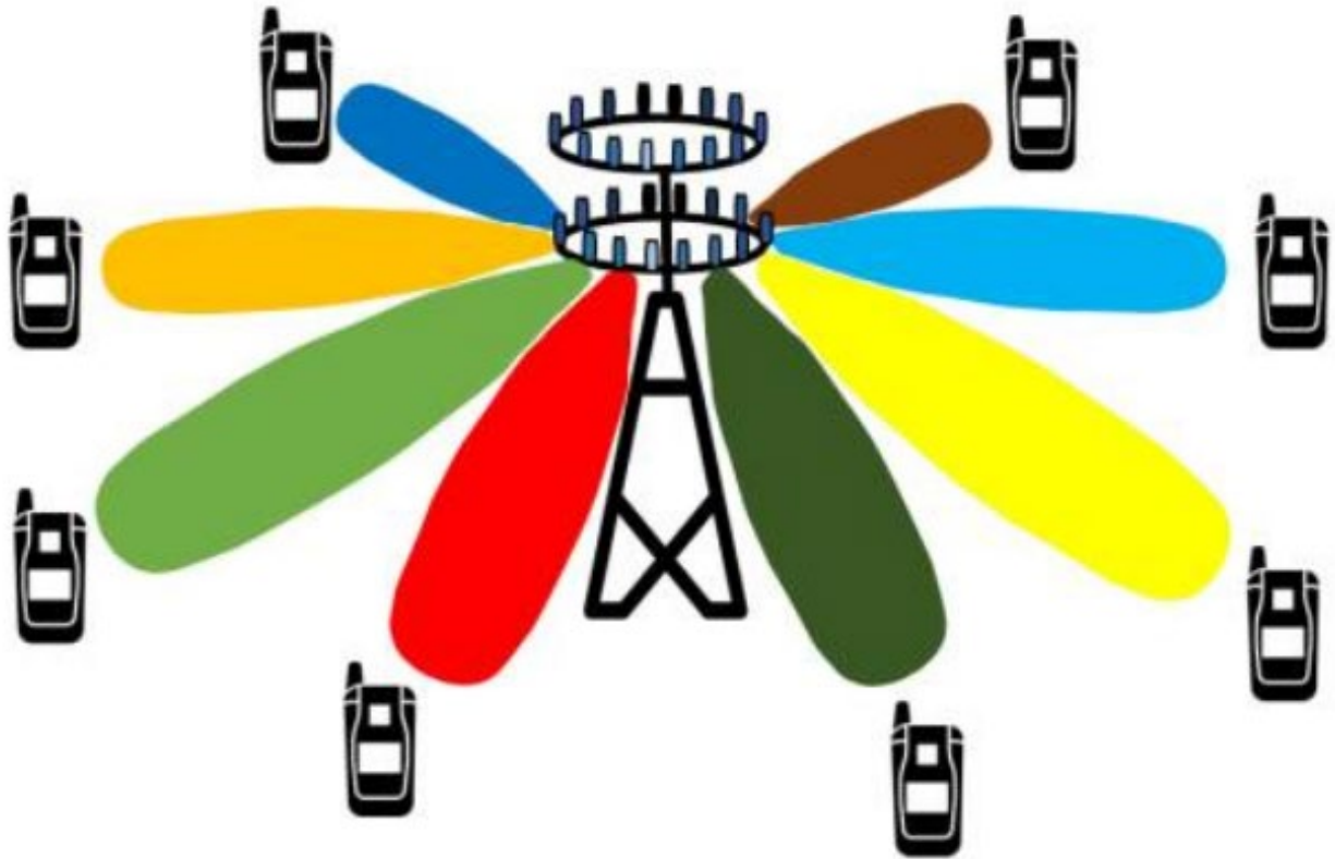
Figure 4: Massive MIMO Beamforming (Source: https://www.ncbi.nlm.nih.gov/pmc/articles/PMC7284607/ ).
